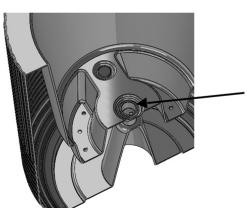
For indoor use, press the red plug down firmly into the overflow drainage hole to seal the planter before use.
